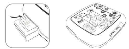
As the battery pack is inserted, the device starts a self-test. If the device status is normal,  $\bigcirc$  is shown on the Status LCD. If  $\mathbf{X}$ ,  $\bigcirc$  or  $\bigcirc$  is displayed on the Status LCD after the self-test, please refer to [Chapter 8: Troubleshooting] of these Instructions for Use.
