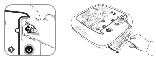
3. Insert the pads connector of the new pads into the Defibrillator Pads Connector , and then put the pads package in the Pads Storage Compartment as illustrated below.
